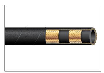
Used for high pressure hydraulic lines on off-road construction equipment, machine tools, **APPLICATIONS:** farm and marine equipment. Meets or exceeds SAE 100R2 and EN 853 2SN.
