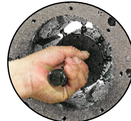
Quick Change Tool Makes die changes a quick and simple process.
