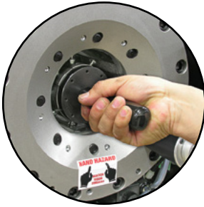
84mm Quick Change Tool (Included) P/N:102572
