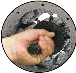
99mm Quick Change Tool (Included) P/N: 102571
