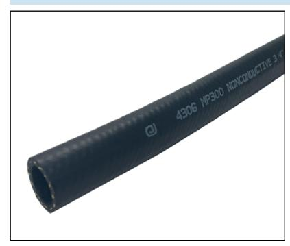
**CONSTRUCTION:** Nitrile ARPM Class A tube, Nitrile blend ARPM Class A cover, 4-spiral polyester yarn
